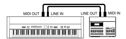
Next you must match the MIDI channel. The transmitting channel of the CA piano and receiving channel of your external MIDI device must be the same.
